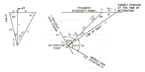
Figure 1. Fragment-target intercept geometry.
