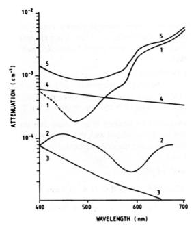
Figure 4. Contribution to total attenuation from different processes.
