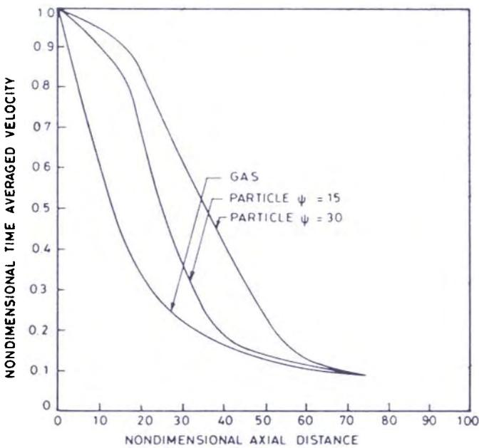
Figure 4. Time-averaged velocity profiles for particle and gas.
