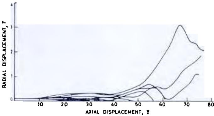
Figure 3. Particle trajectories (random process).
