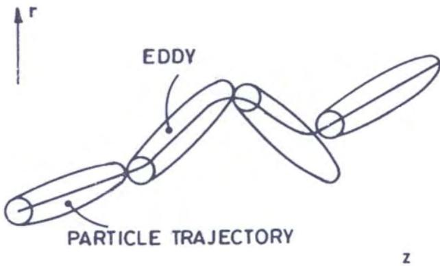
Figure 2. Particle trajectory model.
