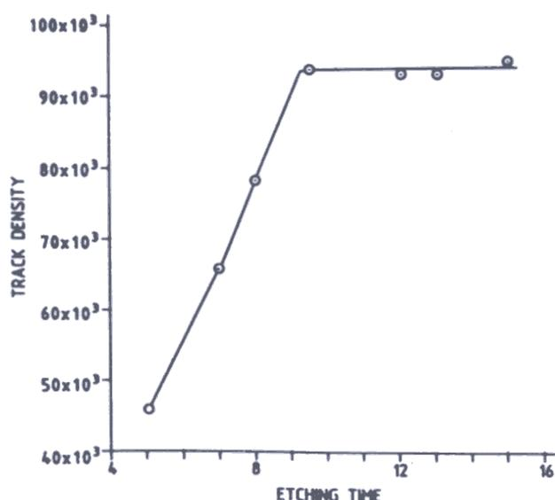
Figure 2. Plot of alpha track density versus etching time.
