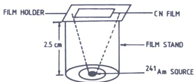
Figure 1. Geometry for exposure of SSNTD films to  $^{241}\text{Am}$  source.
