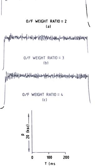
Figure 2. Pressure-time curves for carene-norbornadiene-RFNA at different O/F weight ratios.
