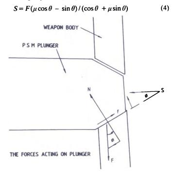
Figure 4. The study of force structure of plunger.
