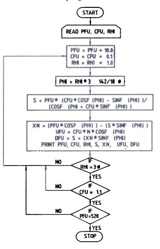
Figure 5. Flow chart of the computer programme PFU: force exerted by parachute, CFU: coeffcient of friction, RHI: semi-angle of plunger, XN: normal reaction, UFU: upward force, DFU: downward force
