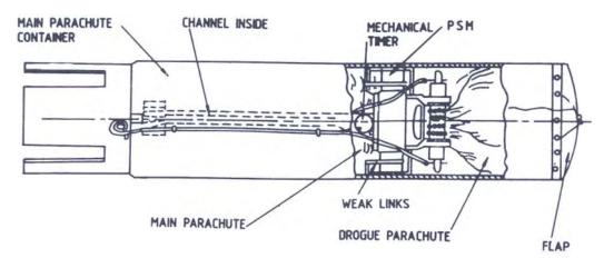
Figure 1. Parachute sequencer
