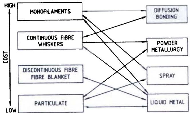
Figure 7. Reinforcement, processing and costs of MMCs for automotive applications.
