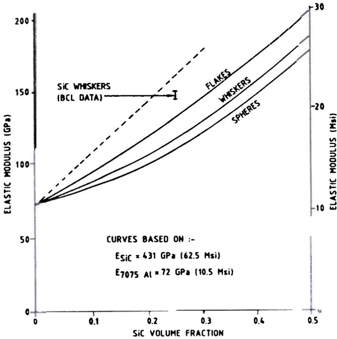
Figure 6. Elastic modulus of SiC-reinforced aluminium alloys.
