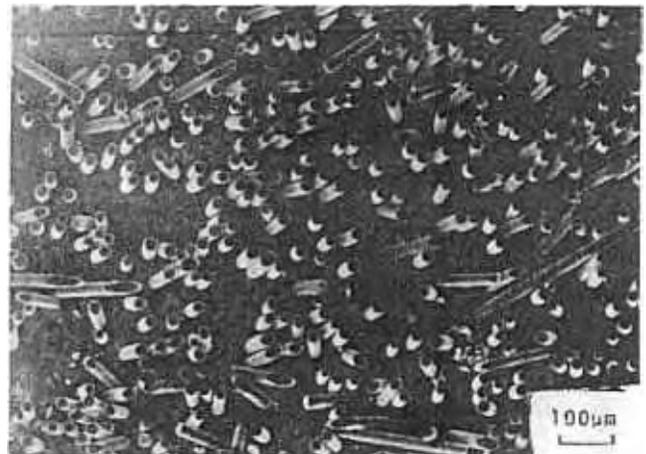
Figure 17. SEM micrograph of electrochemically etched vertical section of cast *Al-4Mg-23* vol % alumina fibre composite showing random planar orientation of fibres (courtesy R. Mehrabian). Mag. 0.96 cm = 150 nm.
