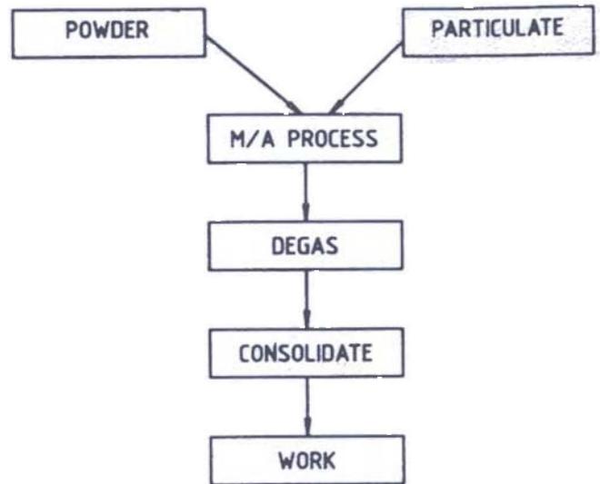
Figure 9. Schematic of the Novamet (Inco mechanically alloyed products) composite preparation process.
