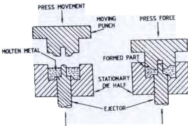
Figure 18. Squeeze casting technique of composite fabrication.
