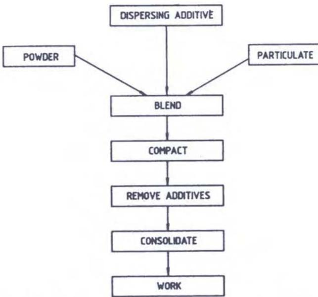
Figure 8. Schematic of the DWA and the Silag composite process (in the Silag process, the 'compact' step is not used).
