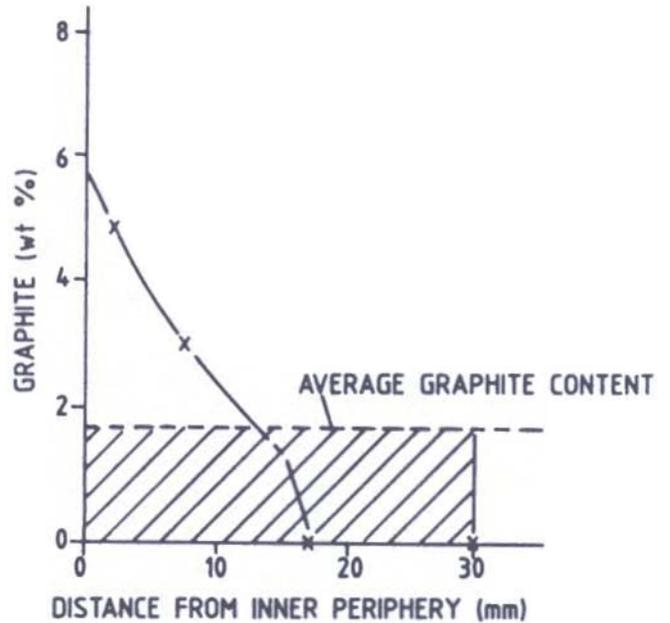
Figure 16. Variation of graphite content with distance from inner periphery of centrifugally cast (average), poured at 710 °C at a speed of 680 rpm.
