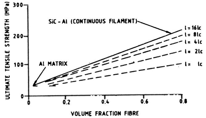
Figure 5. Composite strength as affected by volume loading and whisker length as a multiple of minimum (critical) whisker length for full load transfer.
