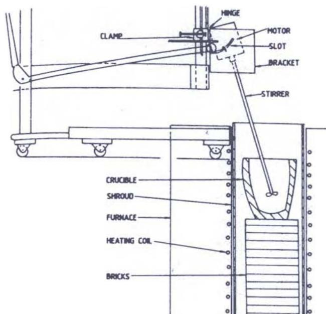
**Figure 11** Schematic of experimental set up to make cast particulate composites.
