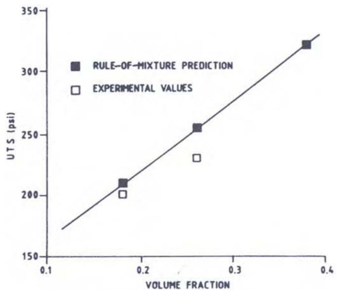
Figure 3. Comparison of the rule-of-mixtures prediction and the observed ultimate tensile strength for an aluminium stainless steel continuous filament-reinforced composite material.
