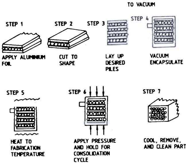
Figure 4. Diffusion bonding process of making fibre-reinforced MMCs.
