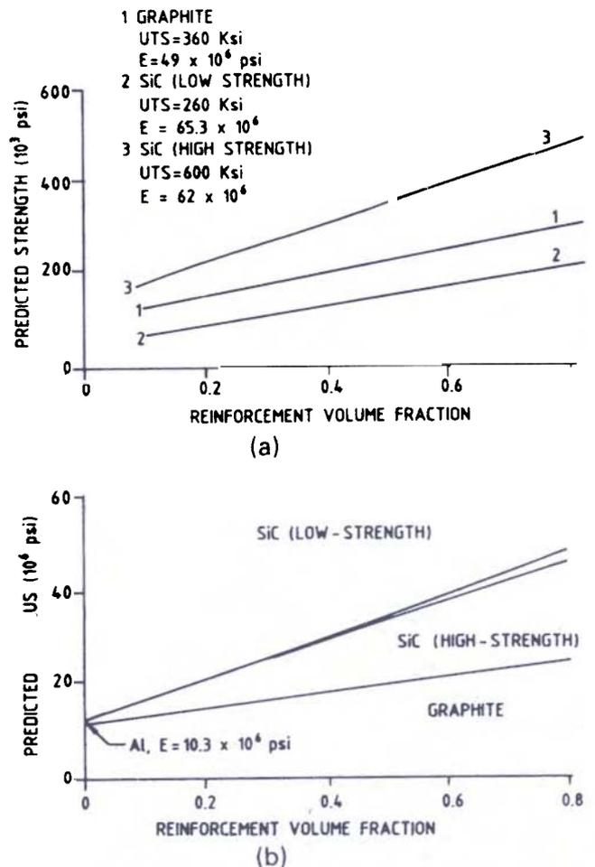
Figure 2. Predicted properties of aluminium matrix composites as a function of filament volume content (a) ultimate tensile strength, and (b) elastic modulus.
