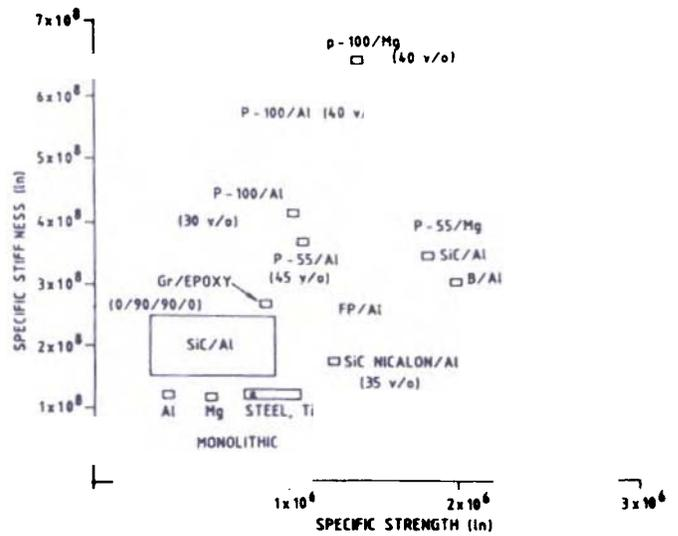
Figure 1 Specific properties of aluminium and magnesium-matrix composite materials, compared to unreinforced alloys (Properties of continuous fibre-reinforced materials are calculated parallel to the fibres).
