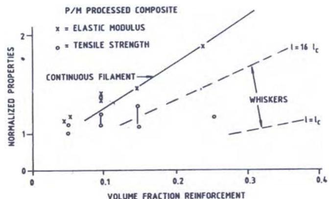
Figure 10. Comparison of normalized values of elastic modulus and ultimate tensile strength vs volume fraction reinforcement in SiC-Al alloys (predicted values for continuous and discontinuous reinforcements are also shown).
