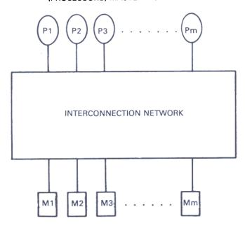
Figure 2. A generalized block diagram of a tightly coupled MIMD machine.
