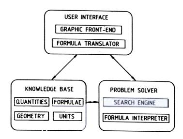
Figure 1. Components of the system.
