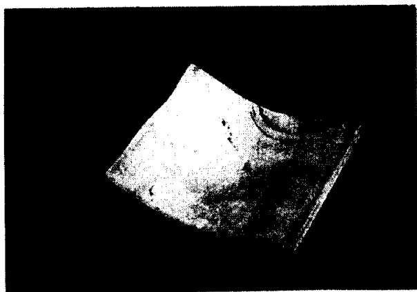
Figure 3b. Buckled bottom plate of 12 mm thickness sandwich in case of no-detonation of sheet explosive with 400 g of donor charge at a distance of 100 mm from the top sandwich plate.
