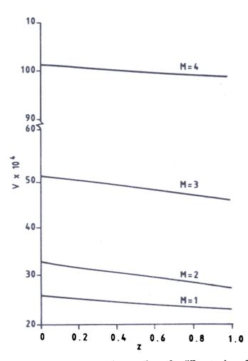
Figure 12. Velocity distribution u against z for different values of magnetic parameter M (case ii).
