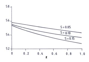
Figure 7. Velocity distribution *u* against *z* for different values of viscoelastic parameter *s* (case ii).
