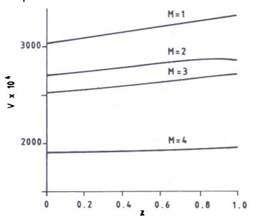
Figure 4. Velocity distribution v against z for different values of magnetic parameter M (case i).
