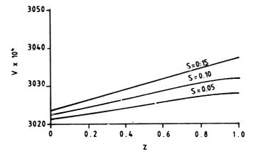
Figure 5. Velocity distribution v against z for different values of viscoelastic parameter s (case i).
