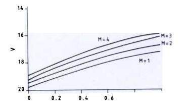
Figure 8. Velocity distribution u against z for different values of magnetic parameter M (case ii).
