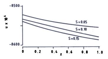
Figure 3. Velocity distribution *u* against *z* for different values of viscoelastic parameter *s* (case i).
