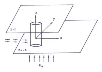
Figure 1 Flow past a circular cylinder.
