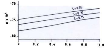
Figure 13. Velocity distribution *u* against *z* for different values of viscoelastic parameter *s* (case iii).
