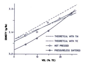
Figure 7. Curve showing density obtained by pressureless and pressure sintering of  $Si_3N_4$ -TiC composites; TiC gets converted<sup>23</sup> into TiN.
