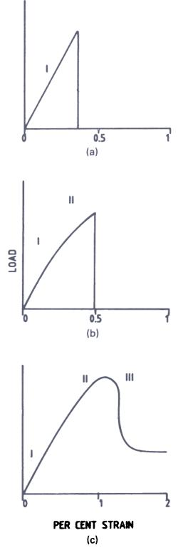
Figure 1. Stress-strain curve for brittle fracture and for composites.
