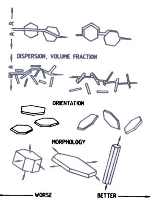
Figure 5. Particle morphology and crack deflection (Telle, R. Brook, R.J. & Petzow, G. J. Hard Materials, 1991, 2, 79-114).
