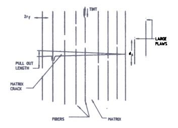
Figure 2. Fibre pull-out during rupture<sup>3</sup>.
