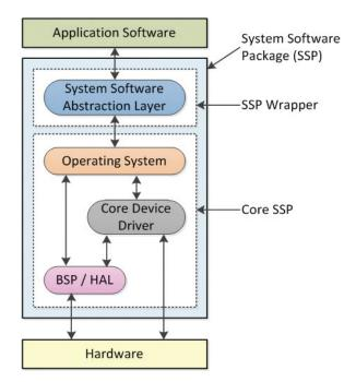
Figure 1. System software package layers.
