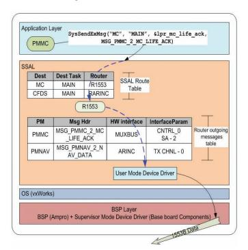
Figure 7. PMMC to MC (driver interface) message transfer through PMR.
