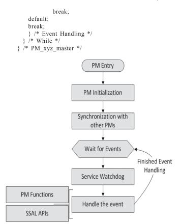
Figure 4. Processing module master thread architecture.
