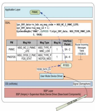
Figure 8. MC to PMMC (driver interface) message transfer through PMR.
