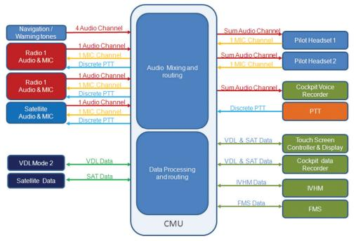
Figure 2. Communication Management Unit interface block diagram.
