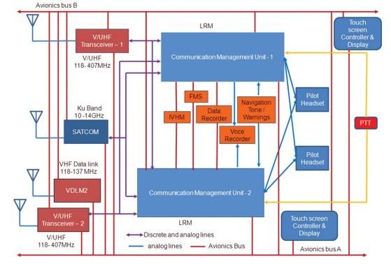
Figure 4. CMU integration on avionics bus.
