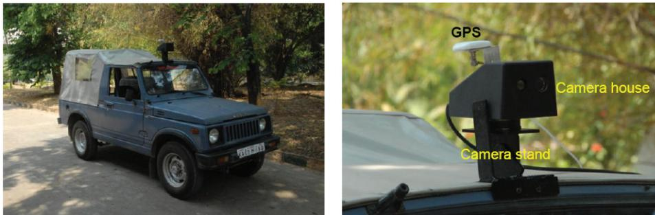
Figure 4. EVS Prototype unit on ground test vehicle.
