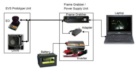
Figure 3. EVS prototype experimental setup.
