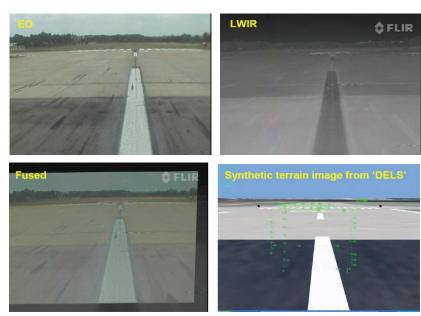
Figure 7. Recorded EO/LWIR, fused and corresponding synthetic image.
