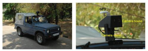
Figure 4. EVS Prototype unit on ground test vehicle.
