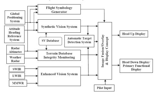
Figure 2. IESVS Subsystem components with other avionic systems.
