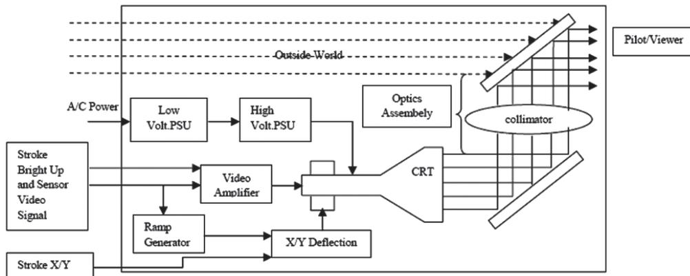
Figure 1. Functional block diagram of hud.
