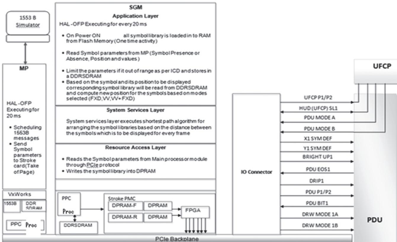
Figure 3. S/W architecture and H/W – S/W interfaces for symbol generation software.
