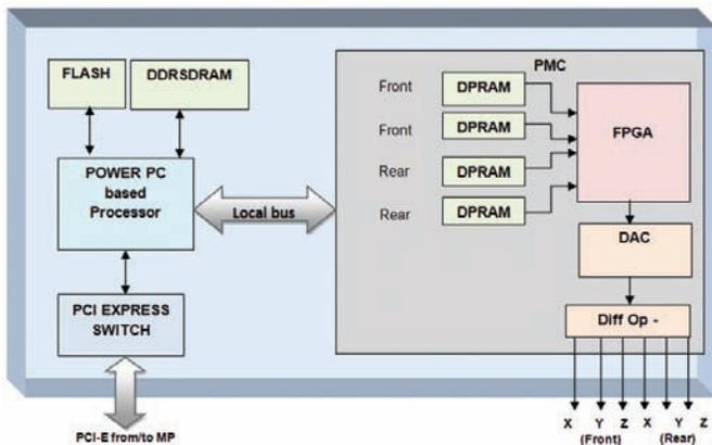
Figure 2. Hardware configuration of symbol generator module.
