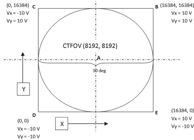
Figure 4. Coordinate mapping on hud.
