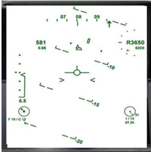
Figure 6. Typical stroke symbols displayed on hud.
