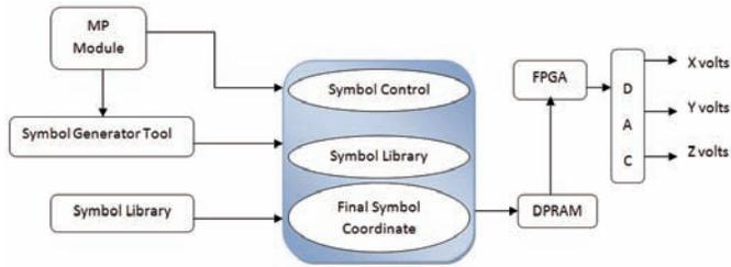
Figure 5. Symbol drawing process.
