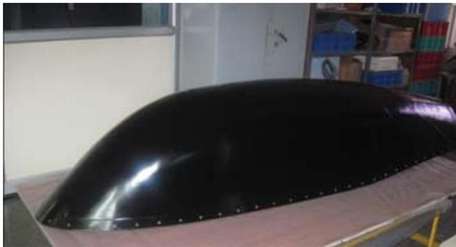
**Figure 15. Lightning protection for SATCOM Radome**
