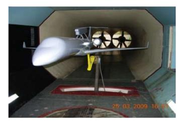
Figure 10. Wind Tunnel Test.
