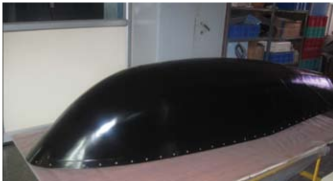
Figure 15. Lightning protection for SATCOM Radome
