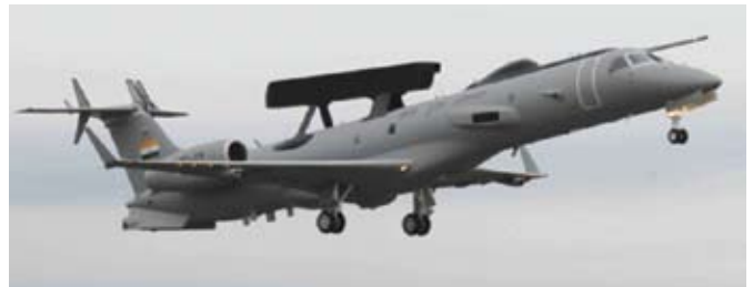
Figure 7. Locating SATCOM Radome and AAAU from aerodynamic and engine considerations.
