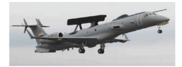
Figure 7. Locating SATCOM Radome and AAAU from aerodynamic and engine considerations.
