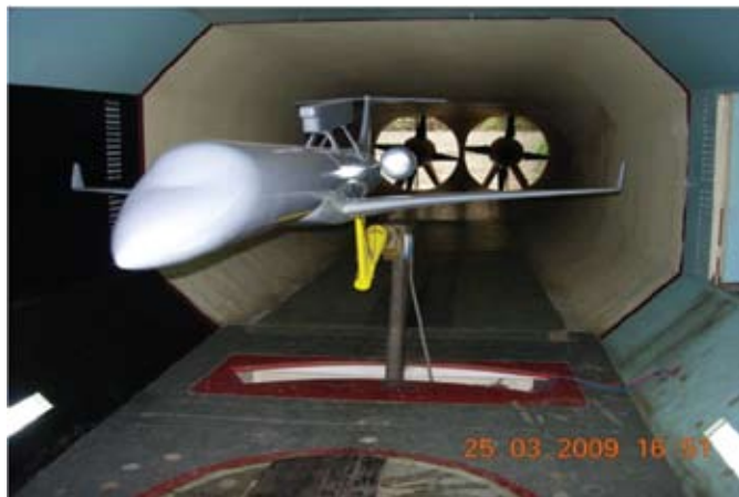
Figure 10. Wind Tunnel Test.
