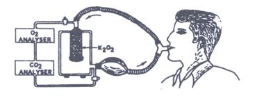
Figure 2. Portable oxygen regenerator set-up.
