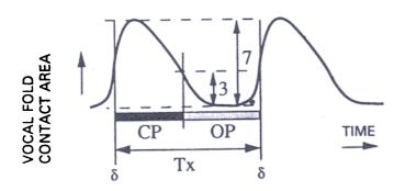
Figure 1. A few cycles of the electrolaryngograph output waveform, showing the measures made to calculate the period (Tx), closed phase (CP), and the open phase (OP).
