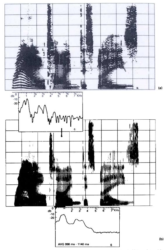
Figure 5. Spectrogram for 'real-time displays' uttered by an adult male, (a) a narrow-band (window length of 512 samples), and (b) a wide-band (window length of 96 samples), along with a short-term (above) and a long-term (below) spectrum in the initial steady portion of the diphthong in 'time' (Calibration: sampling rate: 16 kHz; Y-axis: 1000 Hz/division; X-axis: 250 ms/division).
