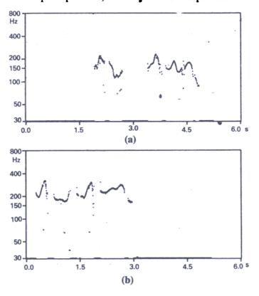
Figure 2. Real-time display of fundamental frequency derived from the electrolaryngograph output waveform for 'he wouldn't say yes, and he wouldn't say no either' uttered by (a) an adult male, and (b) an adult female.
