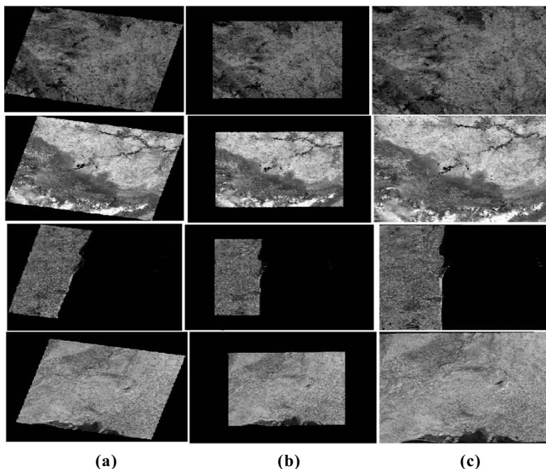
Figure 3. (a) input satellite image; (b) rotated satellite image, and (c) rectified output.
