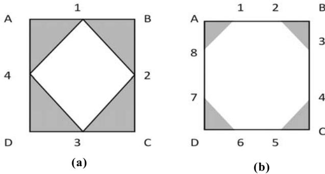
**Figure 1. Distortions of satellite image of a square object in 2-D: (a) with Inclined (row, path), (b) with the IFOV making a polygonal structure with the dark portions filled with zero as entries.**
