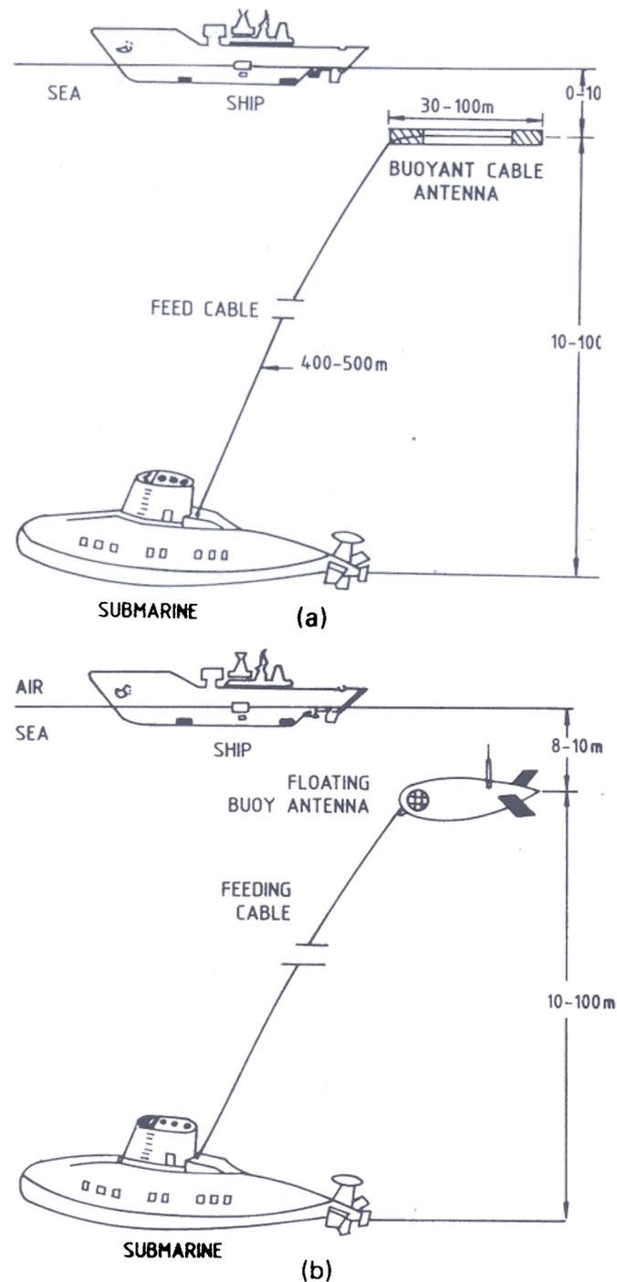
Figure 2. (a) trailing wire antenna, (b) trailing buoy antenna.
