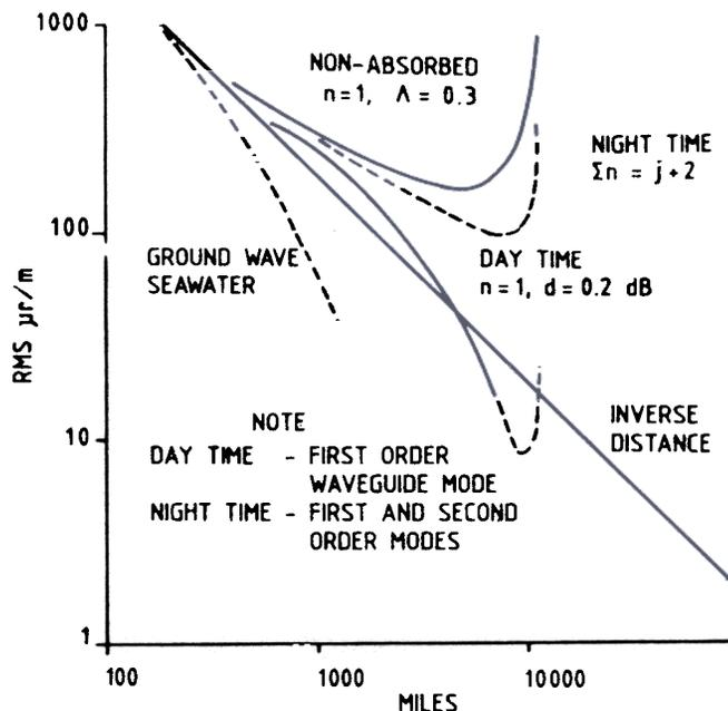
Figure 1. Field strength at various distances.
