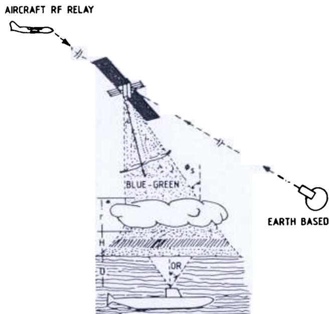
Figure 11. Satellite-based blue-green laser strategic submarine communications system.
