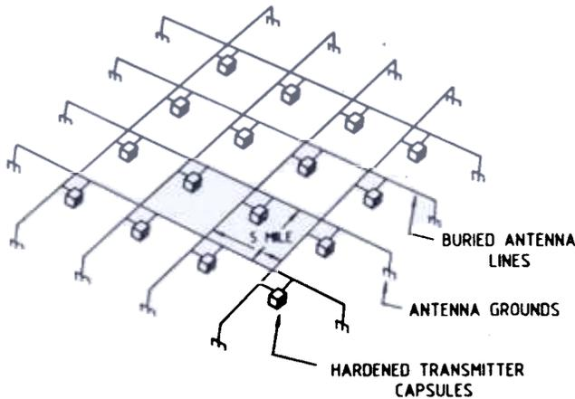
Figure 8. ELF transmitter array.
