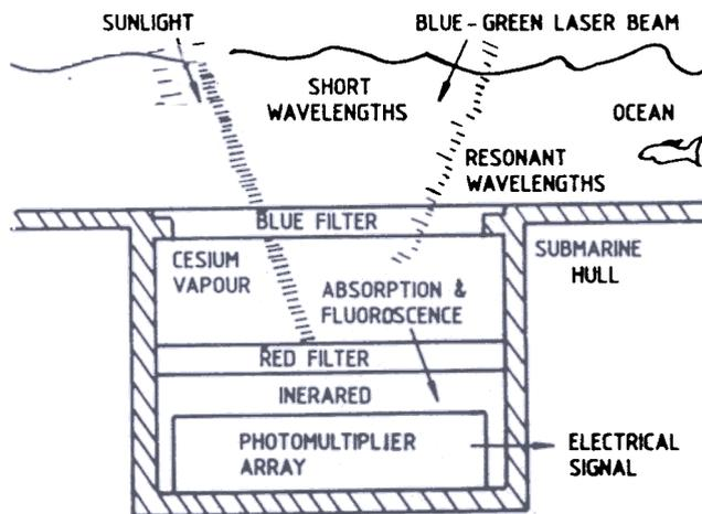
Figure 12. Quantum-limited optical resonance detector.
