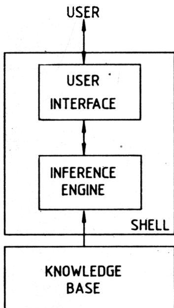
Figure 2. Simplified view of expert system architecture.
