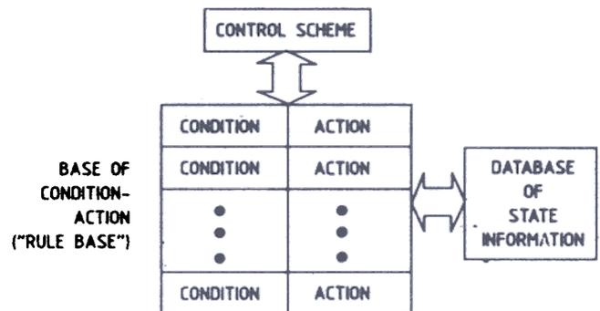
Figure 1. Structure of a condition-action system.
