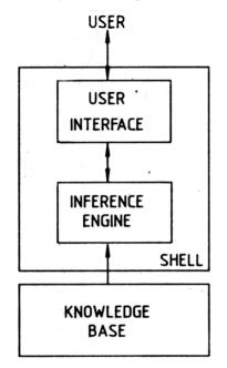
Figure 2. Simplified view of expert system architecture.
