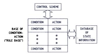
Figure 1. Structure of a condition-action system.
