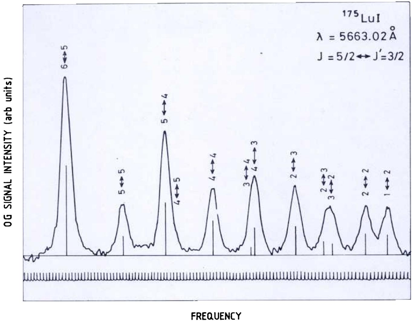
Figure 15. Recorded hyperfine spectrum of  $\text{LuI}$  transition between the high-lying levels  $5d^2 6s^4 P_{3/2} - 6s^2 25p^2 P_{3/2}$  using Doppler-limited LOGS.
