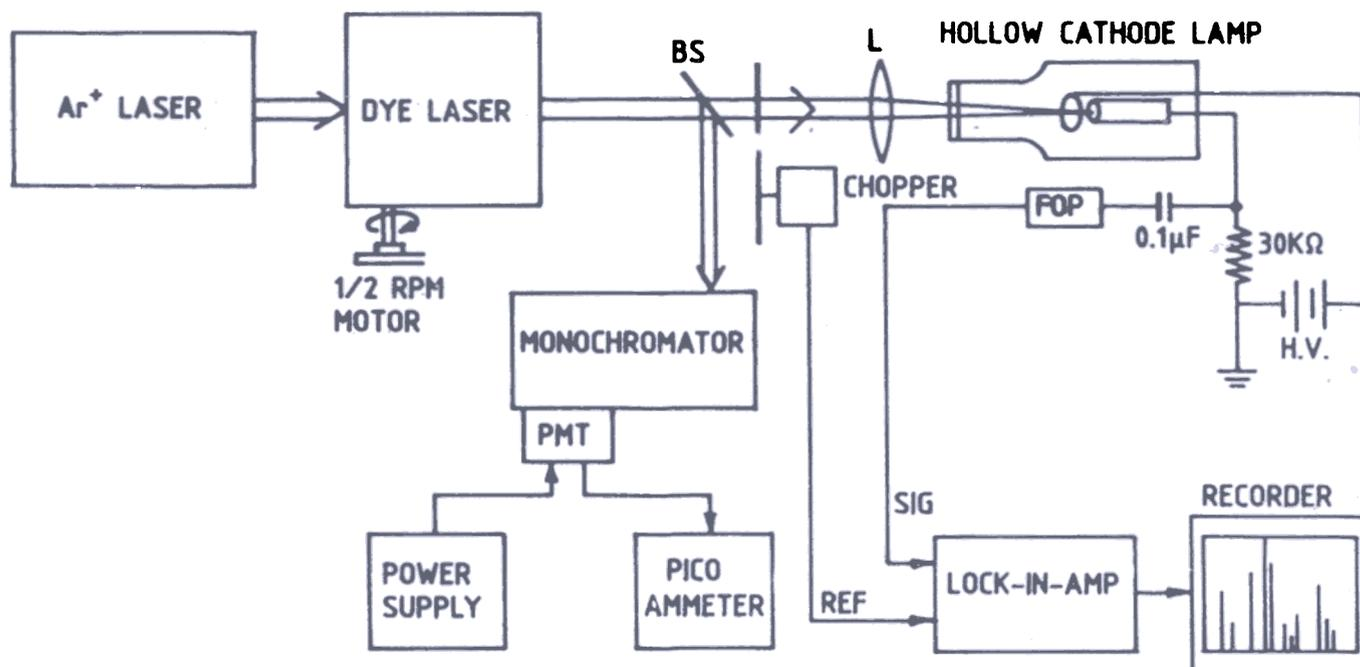
Figure 1 Experimental set-up of LOGS of uranium hollow cathode discharge. FOP-fast overvoltage protection; PMT-photo- multiplier tube
