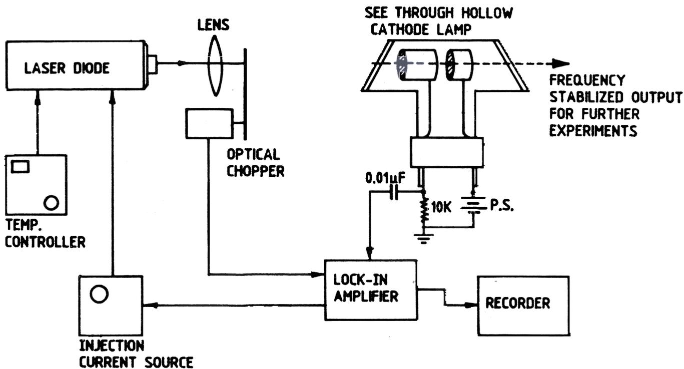
Figure 10. Laser optogalvanic frequency-stabilisation scheme for a semiconductor laser.
