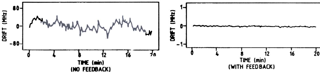
Figure 11. Frequency-stabilised semiconductor laser output
