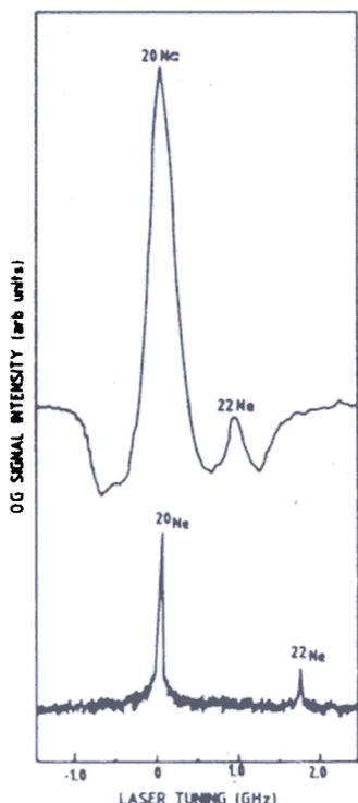
Figure 14. Doppler-free optogalvanic signals of neon for isotope analysis. Frequency scale is different for the two recordings.
