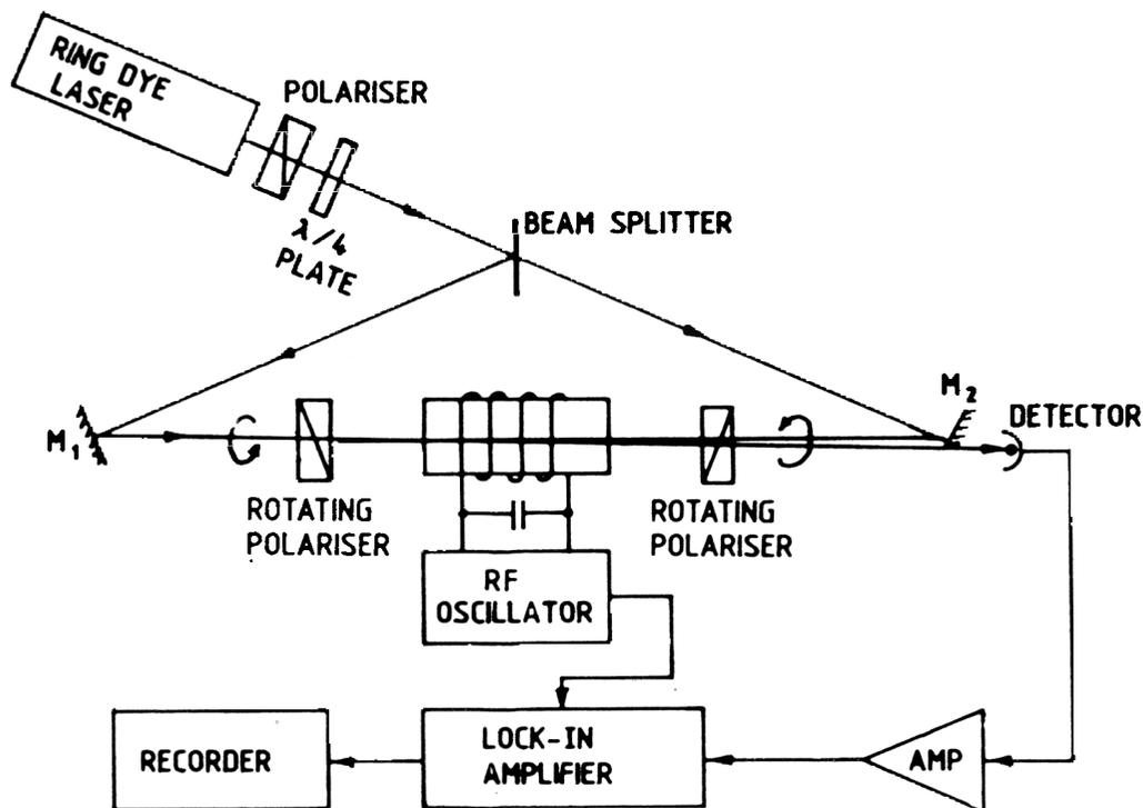
Figure 13. Experimental set-up of POLINEX in RF-discharge.
