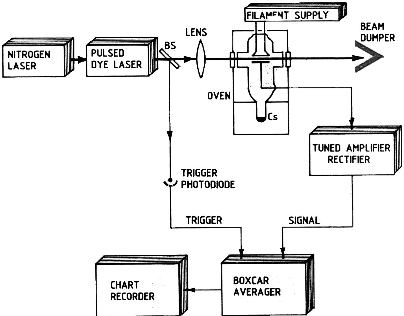
Figure 7. An experimental set-up for thermionic detection of atomic cesium.
