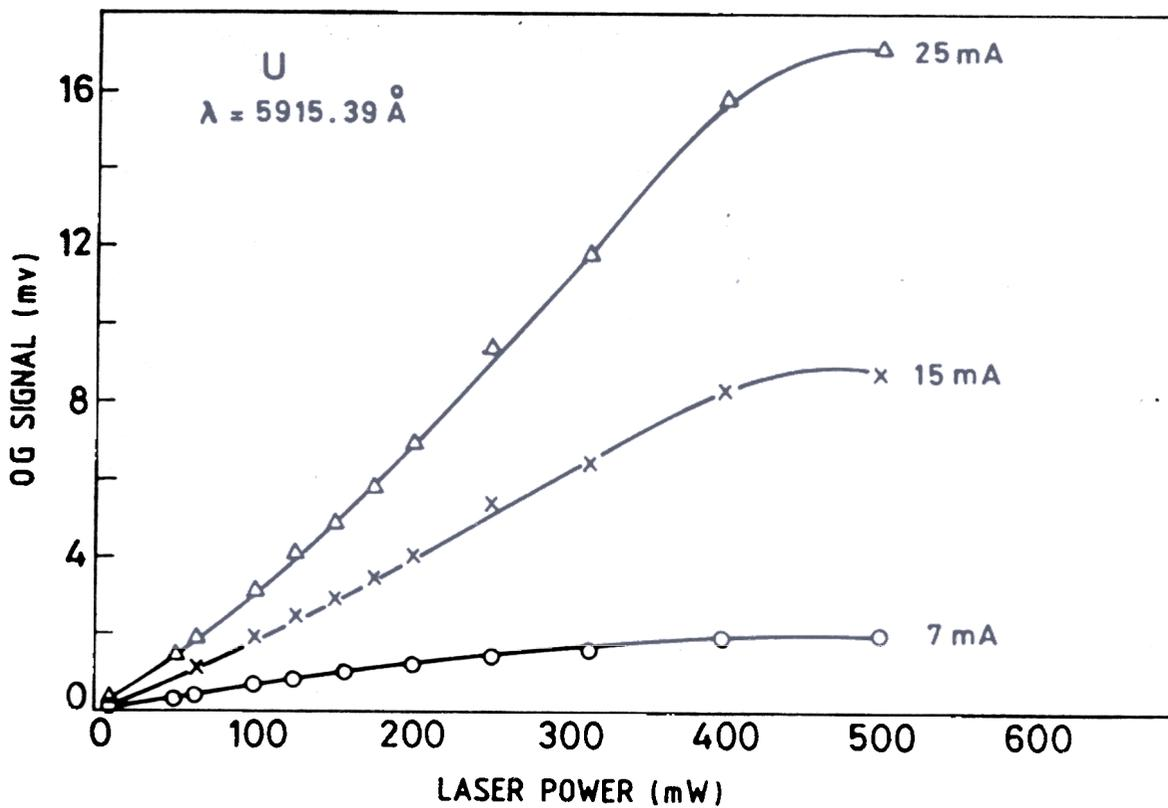
Figure 3. The typical saturation effects of uranium optogalvanic signals in a hollow cathode glow discharge on discharge current and laser power.
