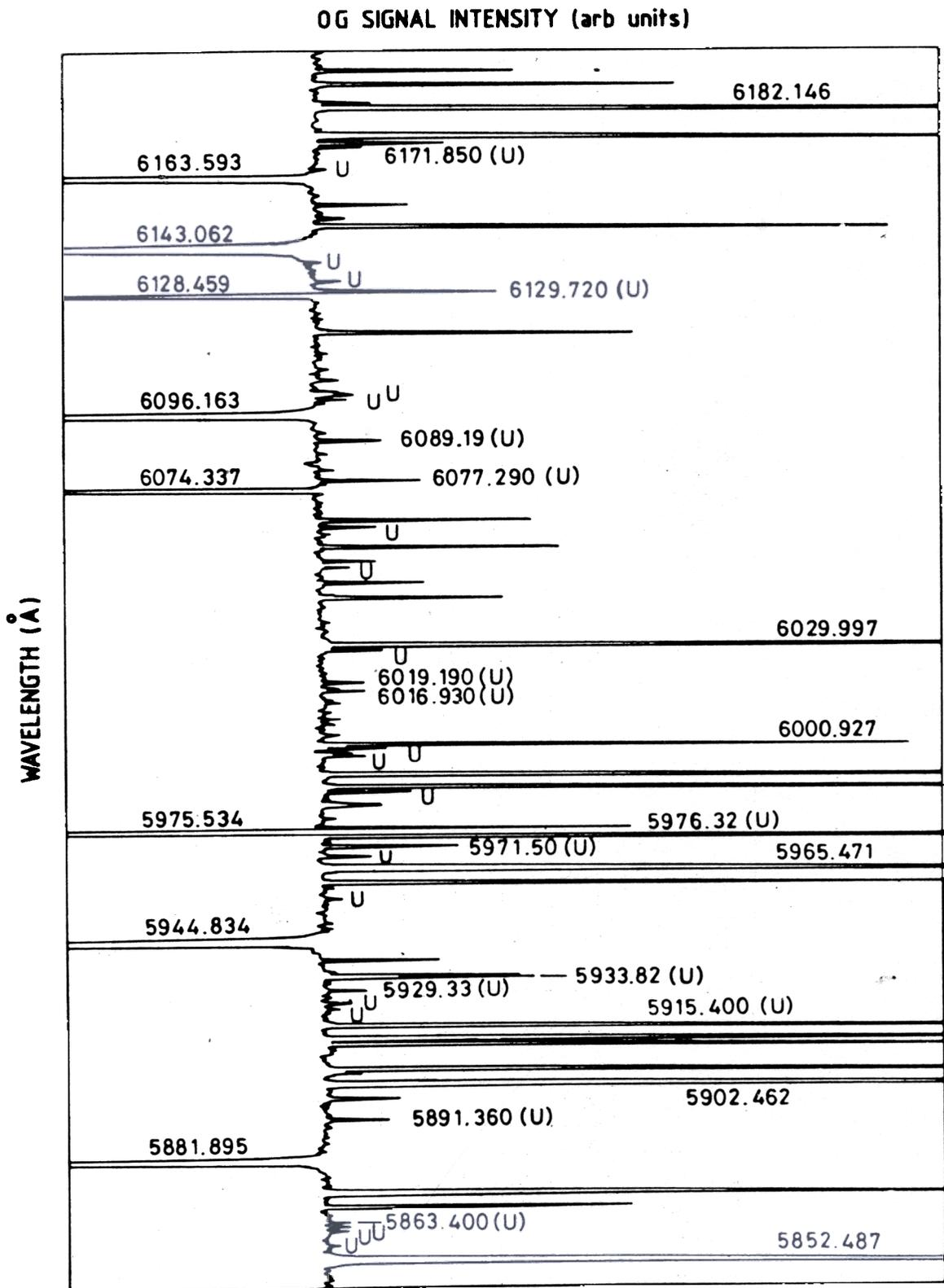
Figure 2. A portion of the recorded optogalvanic spectrum of uranium. Only the strong neon spectral lines used for wavelength calibration are identified.
