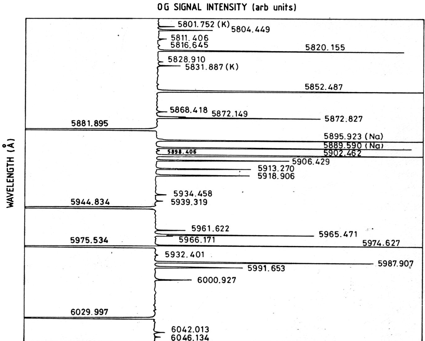
Figure 9. Laser optogalvanic spectrum of sodium-neon hollow cathode lamp. Detection of potassium contamination in pure sodium (99.999 per cent).
