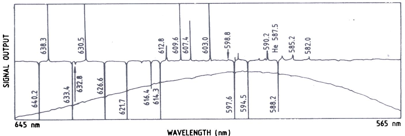
Figure 8. Wavelength calibration of the fluorescence spectrum of Rhodamine 6G dye using broadband optogalvanic spectrum of helium-neon discharge.
