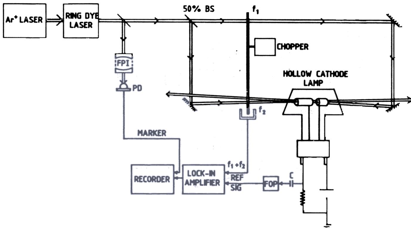
Figure 12. Experimental set-up of IMOGS in a see-through hollow cathode lamp.
