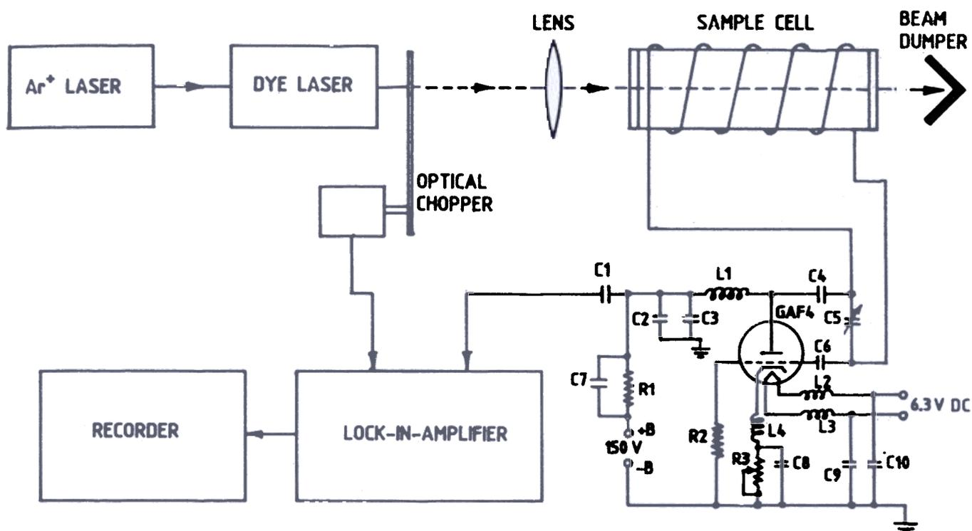
Figure 5. Typical experimental set-up of LOGS on RF-driven discharge.
