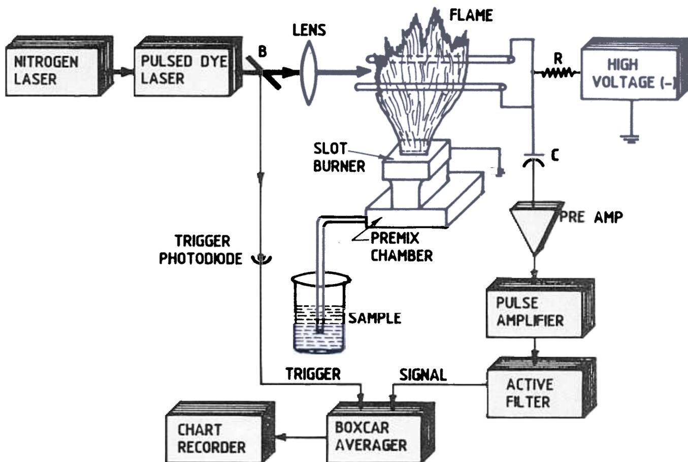
Figure 6. Typical experimental arrangement for pulsed-laser optogalvanic spectroscopy on analytical flames.
