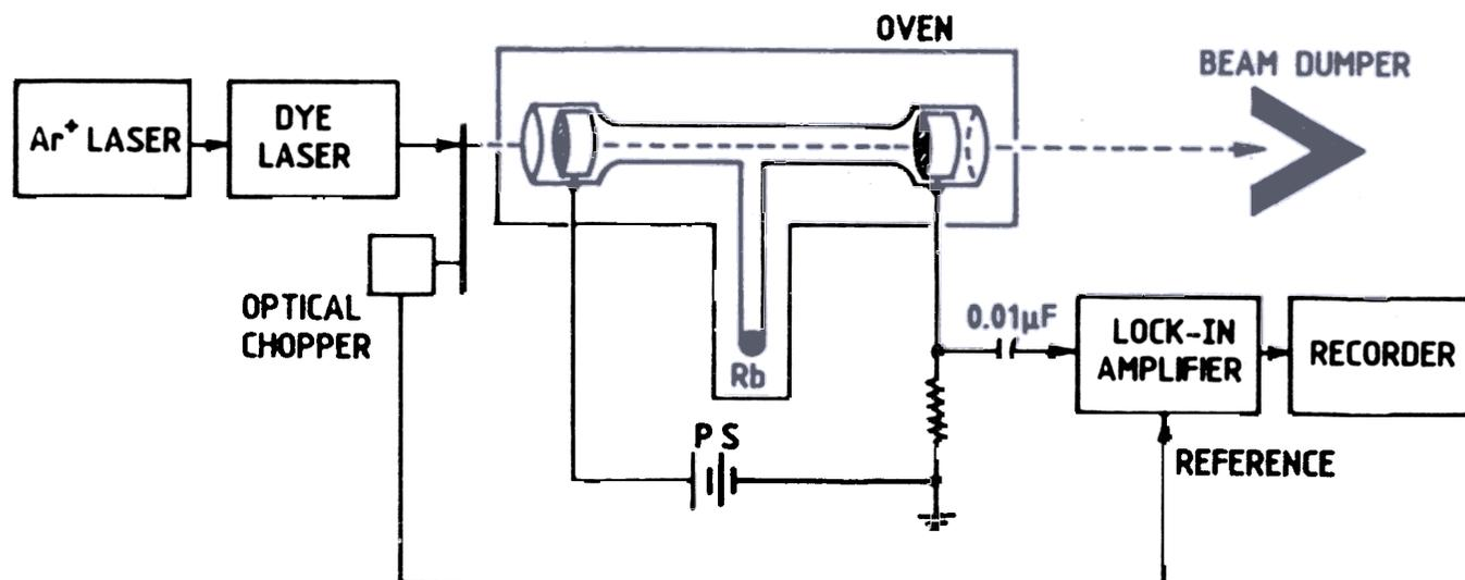
Figure 4. Experimental set-up of LOGS on rubidium positive column discharge.
