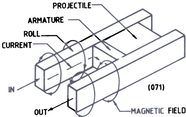
Figure 1. Basic configuration of the railgun.
