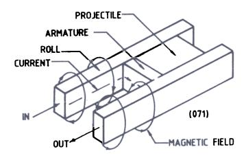
Figure 1 Basic configuration of the railgun
