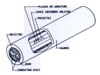
Figure 3. Construction details of the railgun.
