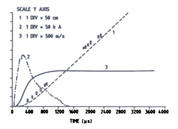
Figure 4. Projectile velocity and displacement computed from the current signal recorded on scopes. The inbore and shorting screen pulses with respect to time are also shown.
