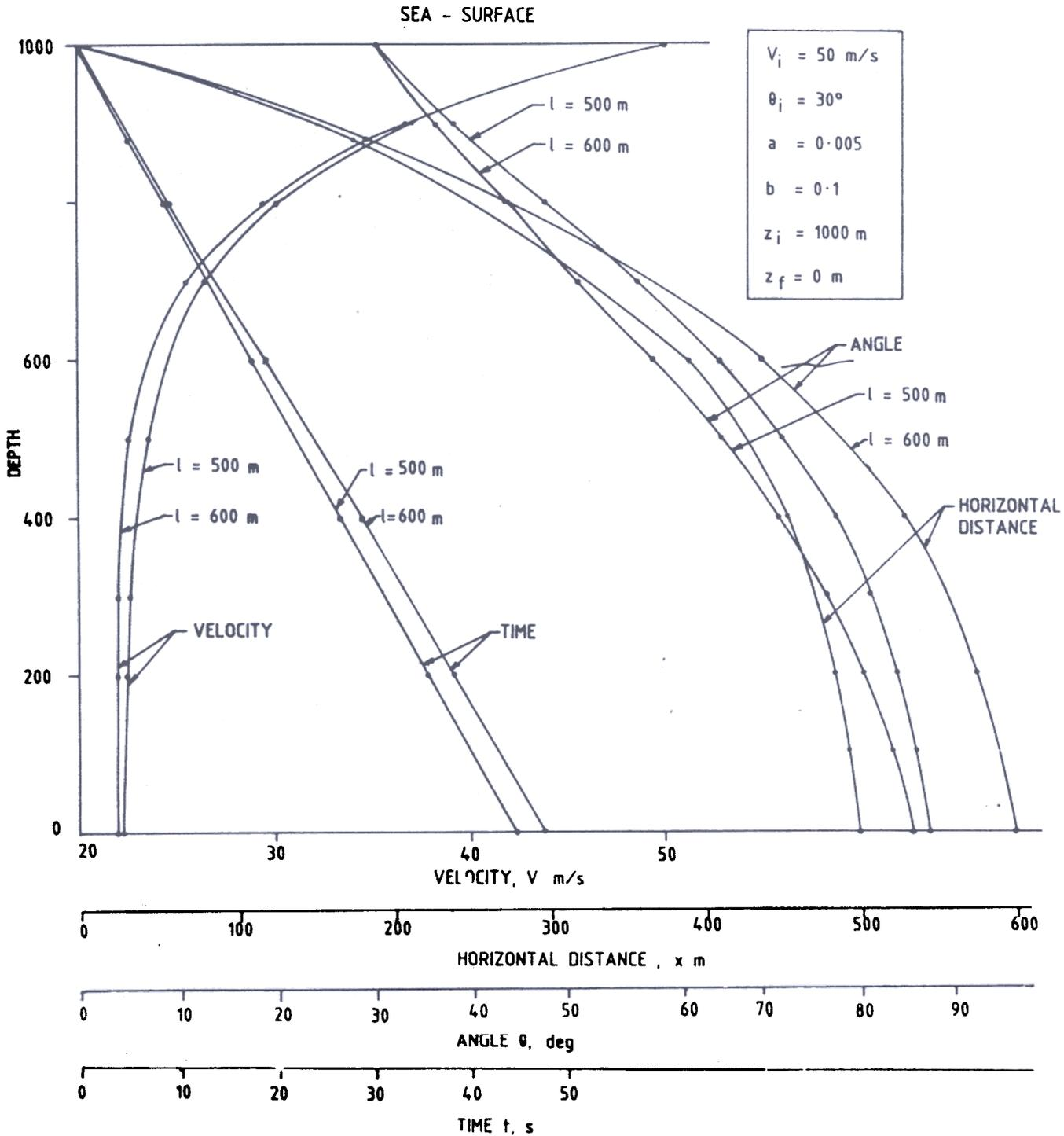
Figure 2. Variation of velocity, horizontal distance, trajectory angle and time with depth.
