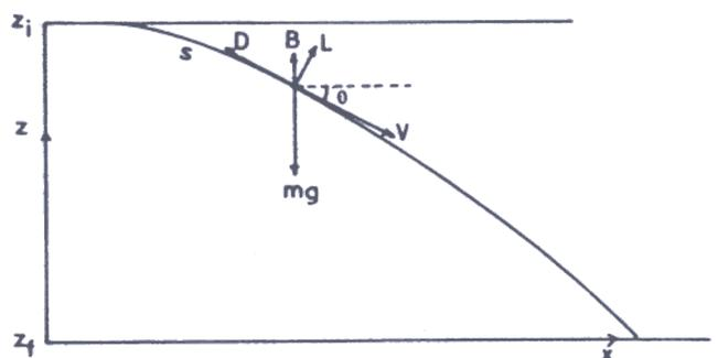
Figure 1. Geometry of the sea-entering vehicle.
