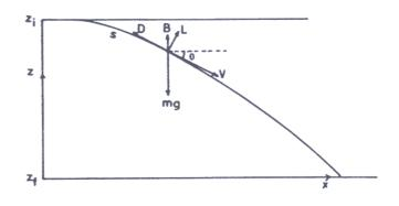
Figure 1. Geometry of the sea-entering vehicle.
