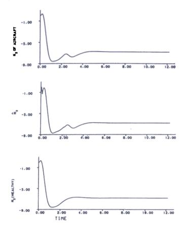
Figure 8.  $N_s$  response with senser failure at 2 s.
