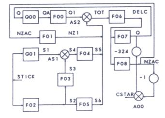
Figure 1 Block diagram of F-8 Cstar controller.
