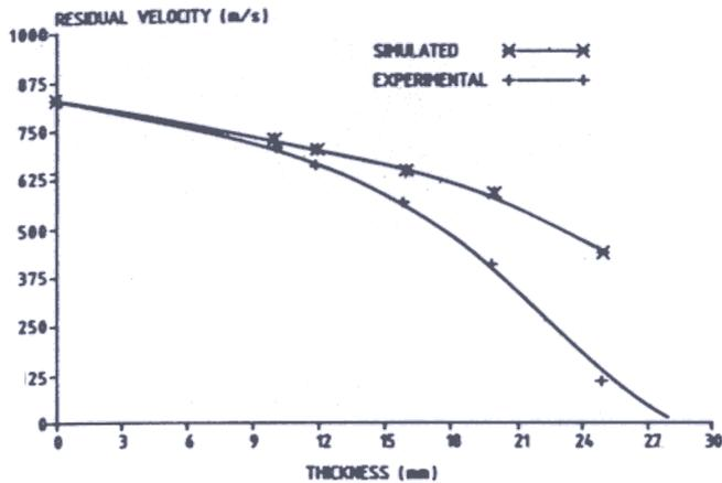
Figure 2. Simulated and experimental results of residual velocity.
