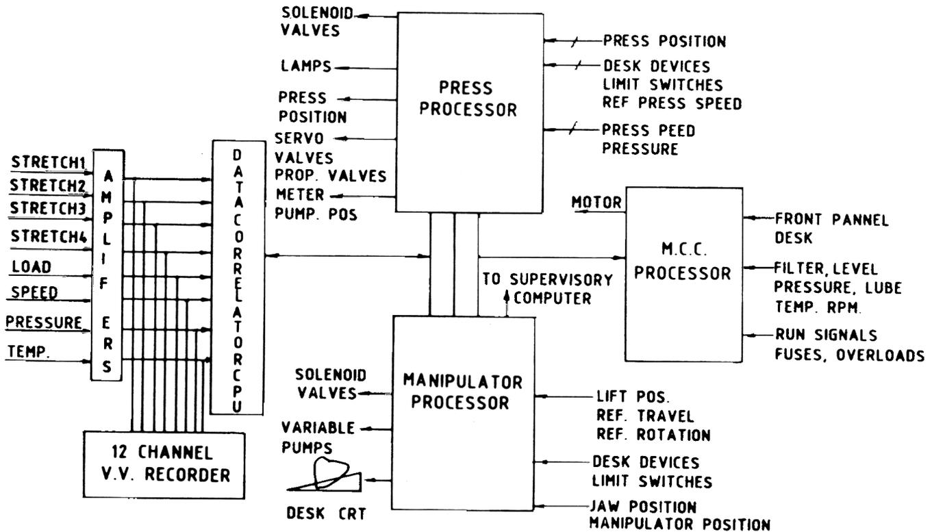
Figure 5. Block diagram of forge press control system.
