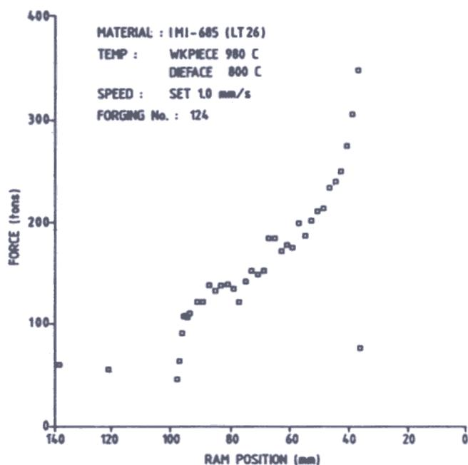
Figure 6. Plot of forging force vs displacement.
