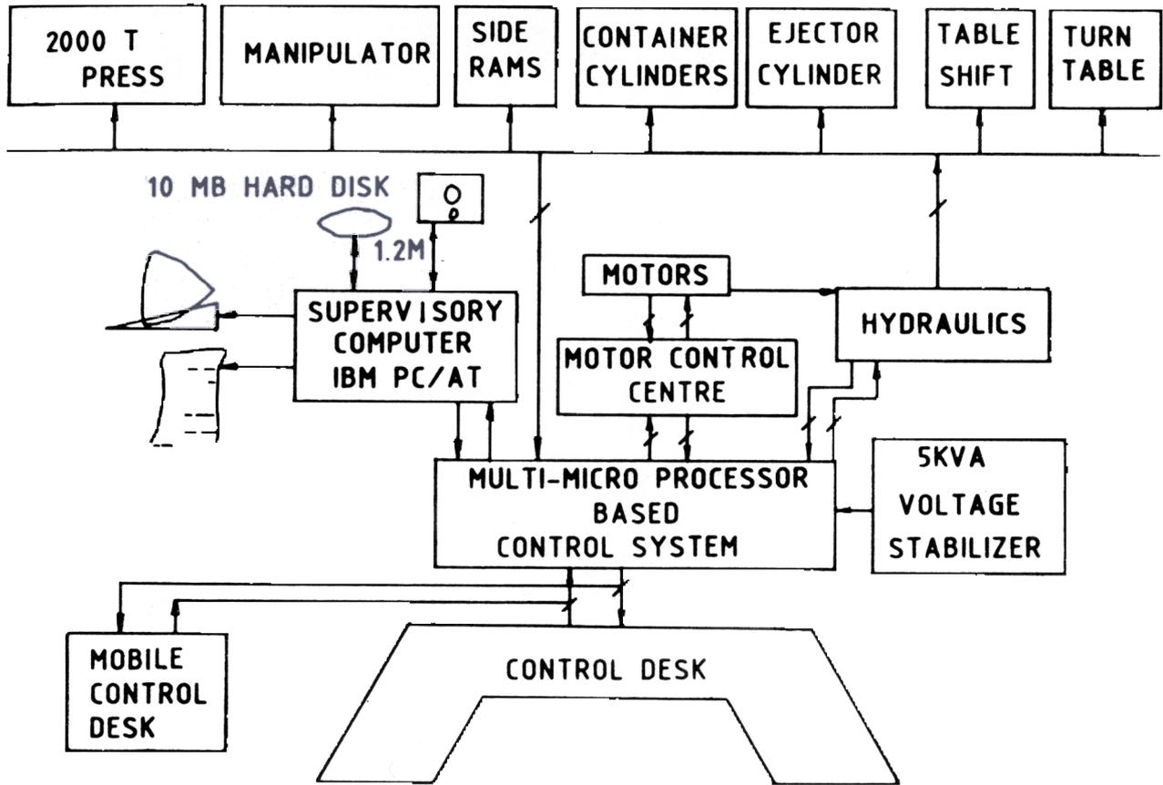
Figure 4. Block diagram of 2000 T forge press.
