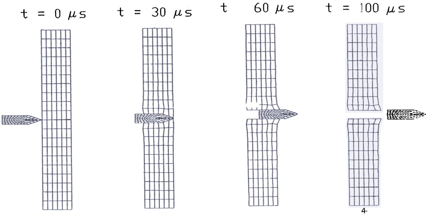
Figure 1 Simulation of penetration at different time steps.
