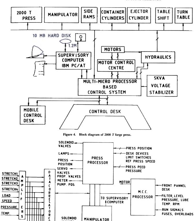
Figure 5. Block diagram of forge press control system.
