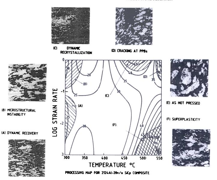
Figure 7. Processing map for 2124 Al- 20v/o SiCp composite.
