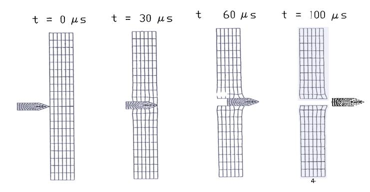
Figure 1 Simulation of penetration at different time steps.
