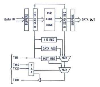
Figure 2. An ASIC VLSI with in-built test access port using boundary scan architecture.
