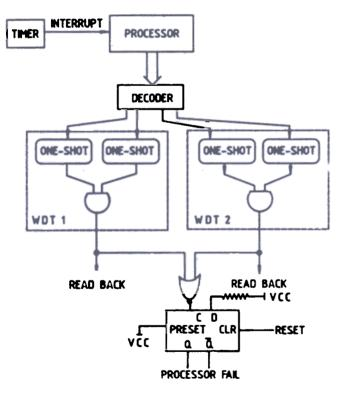
Figure Watchdog timer for detecting processor failure.
