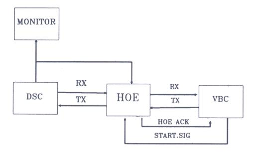
Figure 3(b). HOE interconnection diagram.
