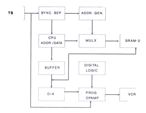
Figure 5. Hardware block diagram for recording HOE performance.
