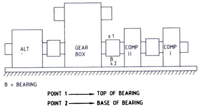
Figure 1 Measurement location of the LP compressor (point 1, top of bearing; point 2, base of bearing).
