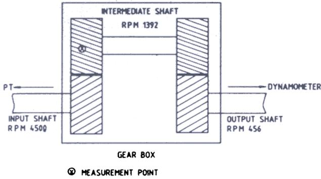
Figure 2. Measurement location of Gearbox ( Measurement point).
