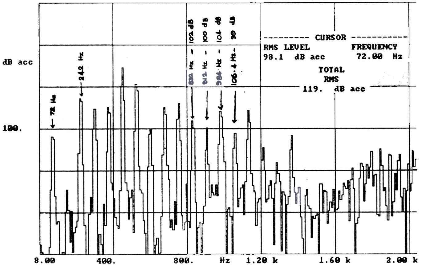
Figure 4(a). LP compressor : Point 2 : spectrum analysis.
