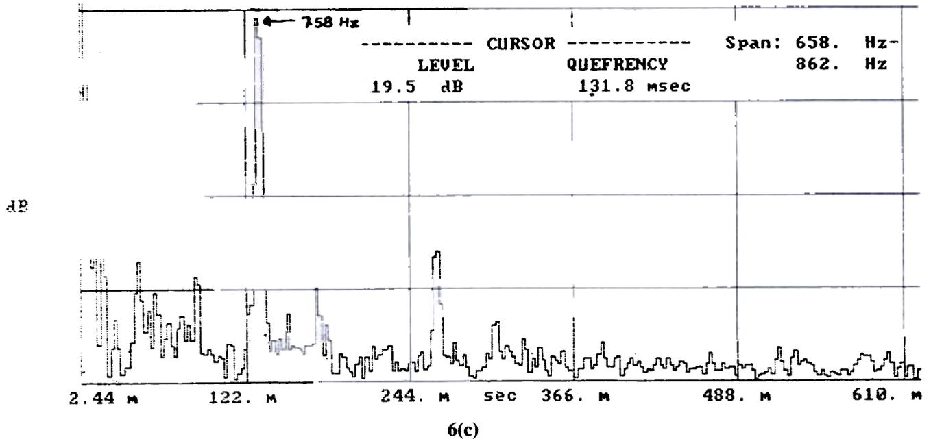
Figure 6. Analyses on the gear box performed at the secondary meshing (76 Hz): (a) spectrum analysis, (b) zoom spectrum analysis, and (c) cepstrum analysis.
