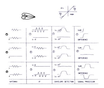
Figure 2. Basic working of the angle tracking system.
