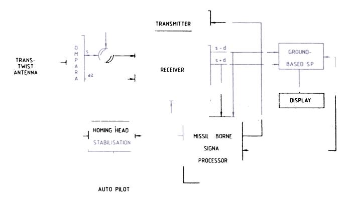
Figure 1. Block diagram of the MMW seeker head.
