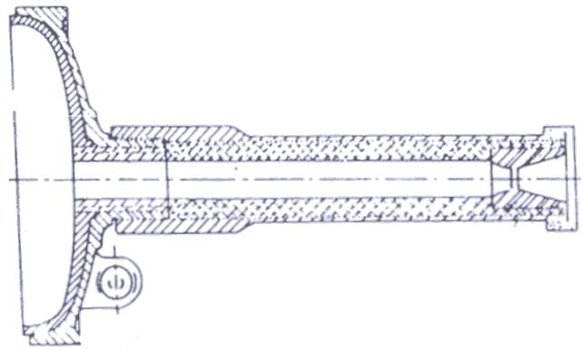
Figure 12. Sustainer nozzle end with subsonic blast tube.
