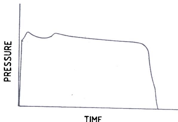
Figure 9. Typical pressure vs time for booster.
