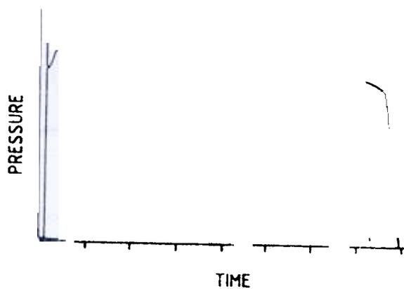
Figure 10. Typical pressure vs time for sustainer.
