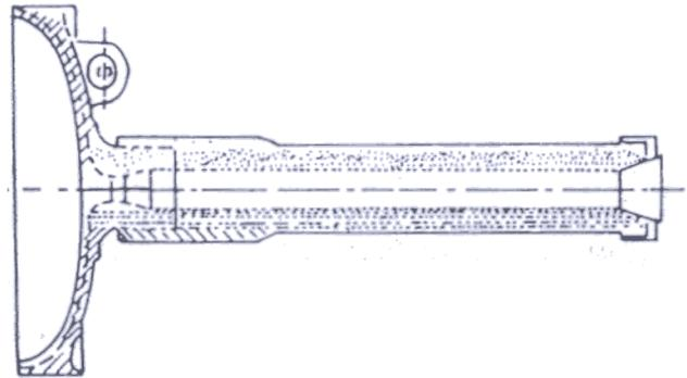
Figure 13. Sustainer nozzle end with supersonic blast tube
