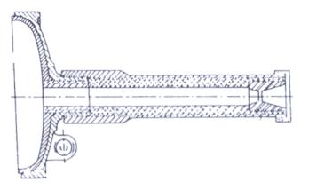
Figure 12. Sustainer nozzle end with subsonic blast tube.
