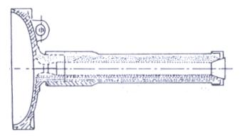
Figure 13. Sustainer nozzle end with supersonic blast tube
