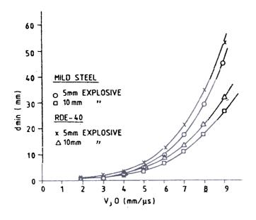
Figure 11 Variation in critical plate thickness ( $D_{min}$ ) with jet tip velocity  $V_j$ o at angle of impact, = 60°.
