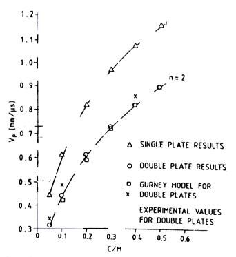
Figure 8. Comparison of the oretical and experimental flyer plat velocities  $U_p$  at different charge to metal mass ratio (c/n in sandwich geometries.
