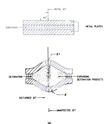
Figure 1. (a) Initial metal explosive assembly, (b) Response of metal-explosive assembly during detonation of explosive.
