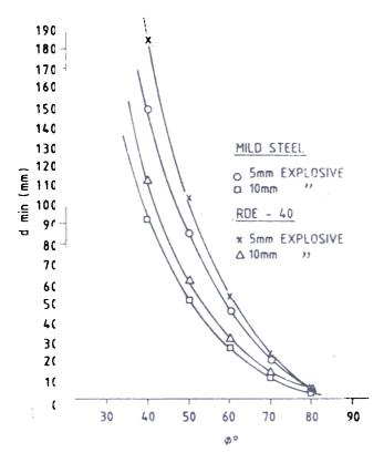
Figure 10. Variation in critical plate thickness  $(D_{olo})$  with angle of jet impact  $(\theta)$  for  $V_j o = 9$ .
