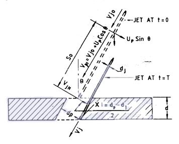
Figure 9. Transvers shifting of jet in moving coordinates during penetration of the plate.
