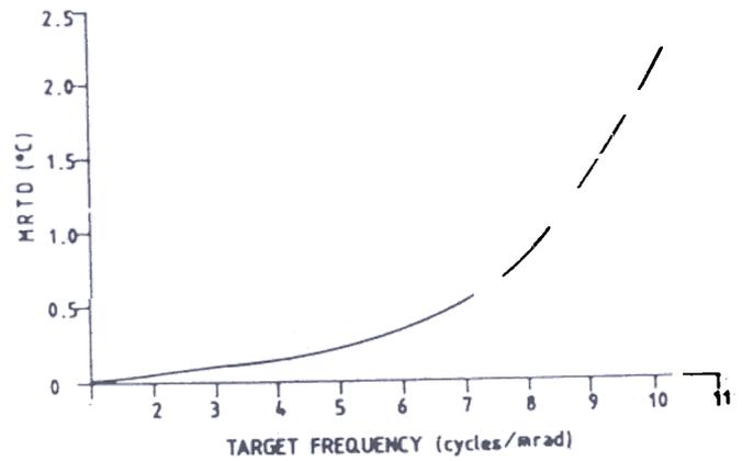
Figure 2. Plot of MRTD vs target spatial frequency.
