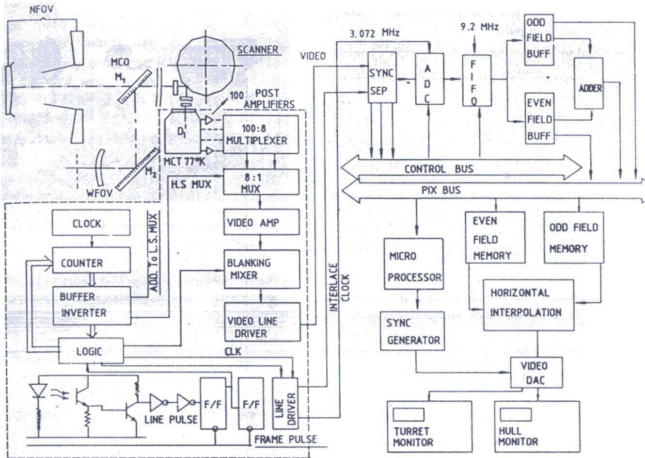
Figure 3. Layout of thermal sight (TS).
