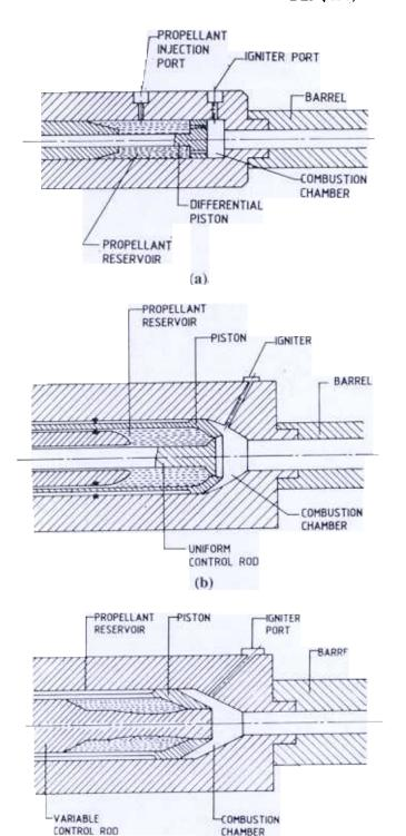
Figure 1 Regenerative liquid propellant guns modelled (a) simple in-line regenerative piston; in-line annular piston with (b) uniform; and (c) variable control rod.
