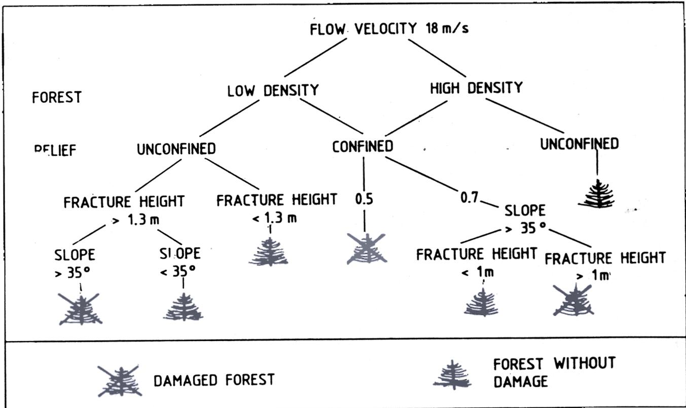
Figure 2. Decision tree for damage to forests for confined and unconfined flows of avalanche (after Gubler and Rychetrik<sup>3</sup>, p.27).
