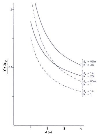
Figure 4. Minimum efficiency of supporting structures for  $\psi = 40^{\circ}$ and  $f_L = 5.8$ .
