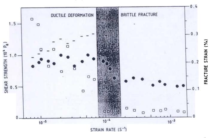
Figure 1. Strain-rate dependence of fracture strain (□), fracture stress (•) and hardening limit stress (—) (after Fukuzawa and Narita<sup>3</sup>).
