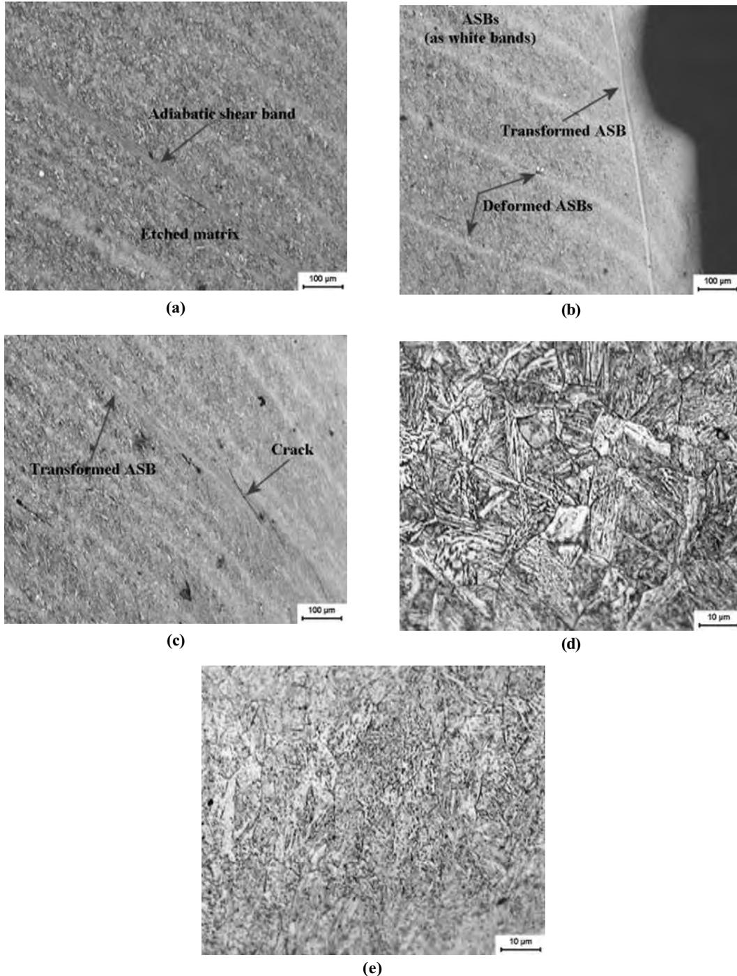
**Figure 3.** The microstructures of the regions marked with alphabetical characters on the macroimage in Fig. 2: (a) The structure of adiabatic shear band (ASB), (b) deformed and transformed ASBs as white bands, (c) the formation of crack-induced ASBs in the matrix, (d) the microstructure of original matrix, and (e) degenerated microstructure close to penetration.
