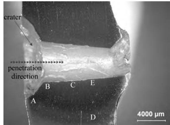
**Figure 2. A macroimage of the cross-section of the perforated zone after the shot.**
