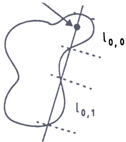
Figure 12. In this figure the measuring line intercepts the same grain several times;  $l_{0,0}$  is the segment of the line passing through the grid point. Other segments of the line intersecting the grain are labelled  $l_{0,i}$ . In the figure  $i = 1$ .
