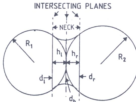
Figure 3. Cross-section through a bonded grain pair.  $R_1$  and  $R_2$  are the grain radii. Neck is the region between the two planes intersecting the grains at a distance  $h_l$  and  $h_r$  from the bond.  $d_l$  and  $d_r$  are the diameters of the neck ends and  $d_b$  is that of the bond.
