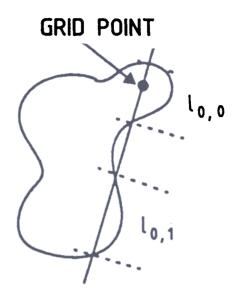
Figure 12. In this figure the measuring line intercepts the same grain several times;  $I_{0,0}$  is the segment of the line passing through the grid point. Other segments of the line intersecting the grain are labelled  $I_{0,i}$ . In the figure i = 1.
