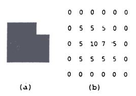
Figure 9. The distance map of Fig. 9(a), generated by Eqns (22) and (23), is shown in Fig. 9(b).
