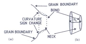
Figure 4. Two and three-dimensional neck configurations. The dotted lines forming a trapezoid are the cross-section of a neck as seen on a surface section. It is generated by determining the corresponding corner points lying on the surface boundary.
