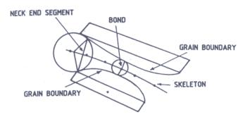
Figure 1 Skeleton and maximal disks corresponding to the bond and end segment of the left half neck.
