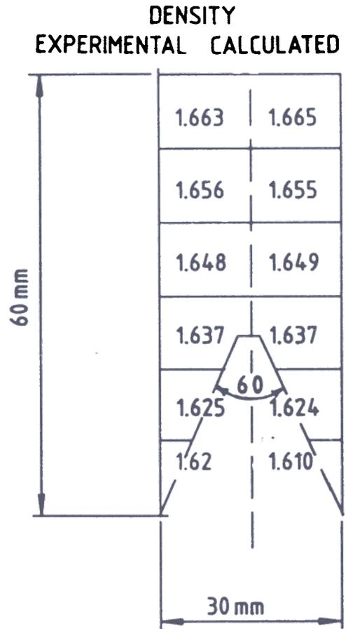
Figure 1. Comparison of calculated and experimental density variation in cylindrical charge.
