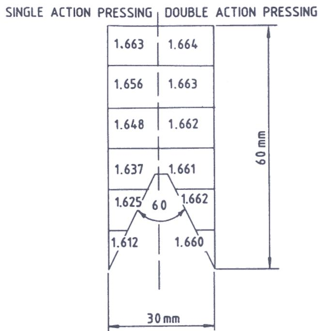
Figure 3. Comparison of density variation by the two pressing techniques.
