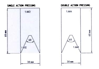
Figure 2. Variation in density between top and bottom in single and double action pressing methods.
