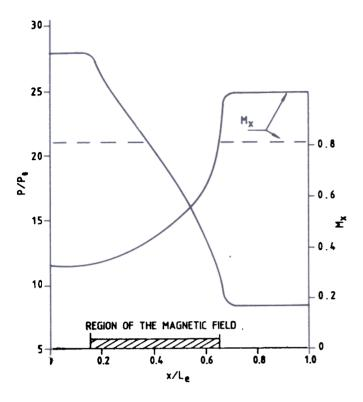
Figure 2. Typical stationary distribution of flow parameters.
