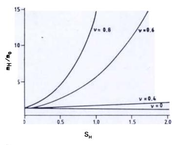
Figure 3. Influence of  $S_H$  and v on relative mass burning rate of solid propellant.
